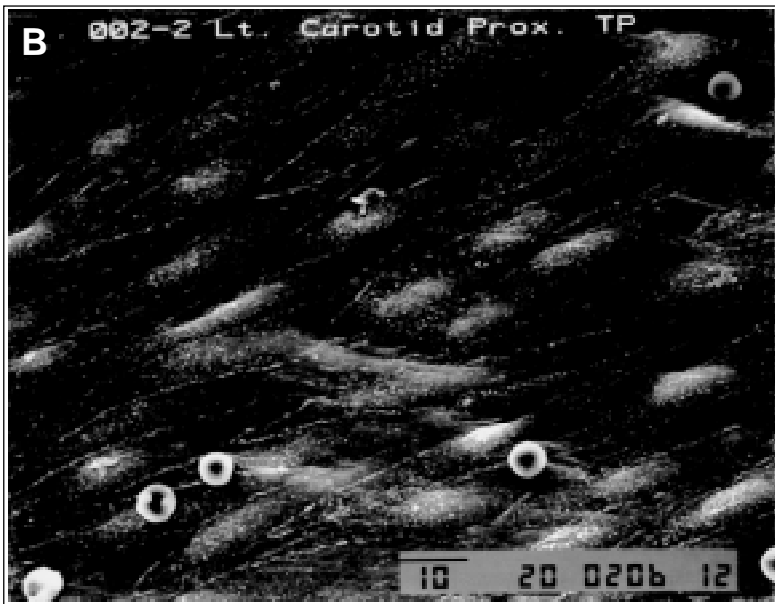
Figs. 8.6A,B. Scanning electron micrograph of luminal side of explanted A) uncoated PET and B) coated PET vascular patch.
